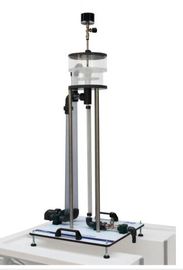
The goal of this equipment is to try to reproduce the experiment by Osborne Reynolds visualizing laminar, turbulent and transitional setting the Reynolds number corresponding to each flow.
